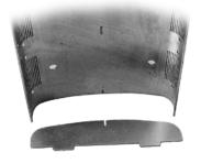
Side bends are now excessively tight so clamp sides (bottom flat 1mm) in vice jaws & ease up slightly to match support rib profile.
